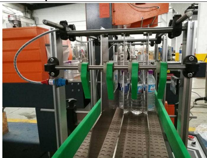
Full piece bottle inlet belt chain to suit all kinds of bottles
