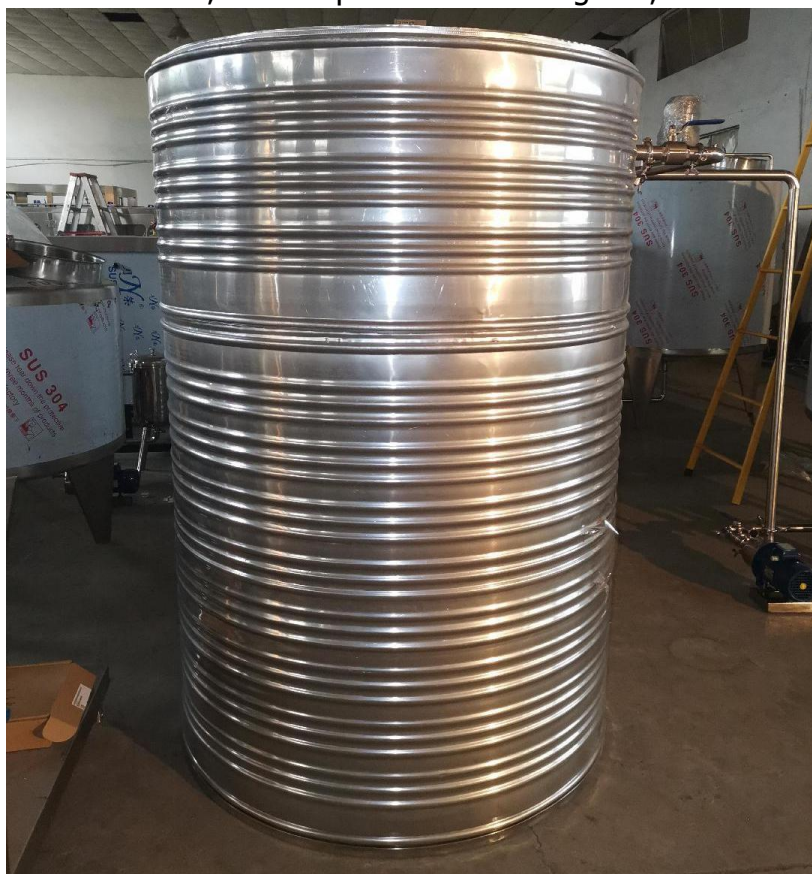
4000L Raw water tank
