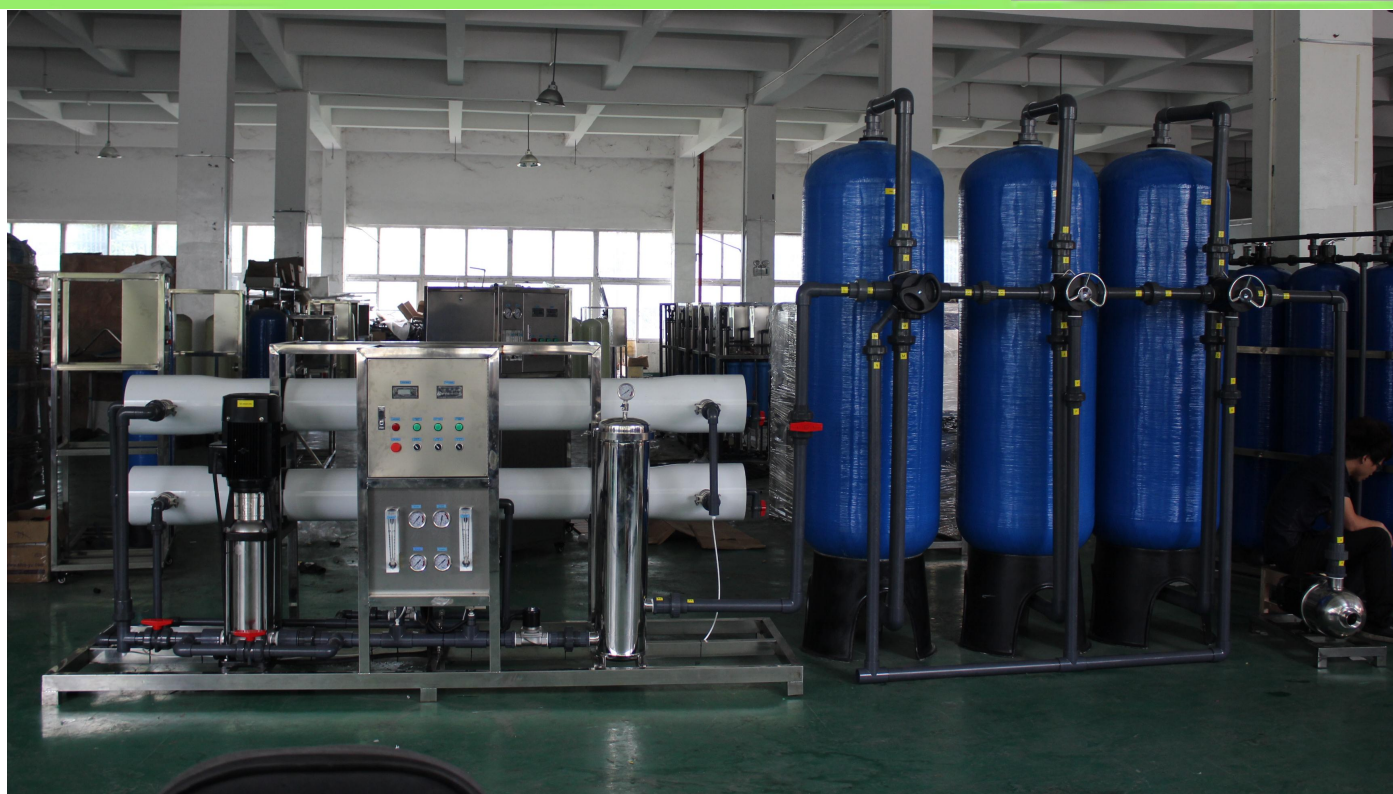
4000LPH RO water treatment machine with 3 filter tanks just for ref.
