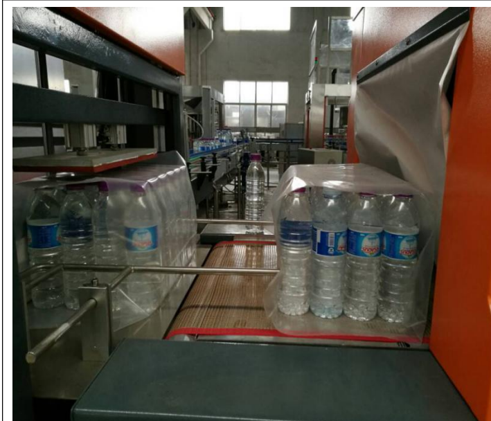
Whole piece bottle pack transmission board to make sure transmission stability
