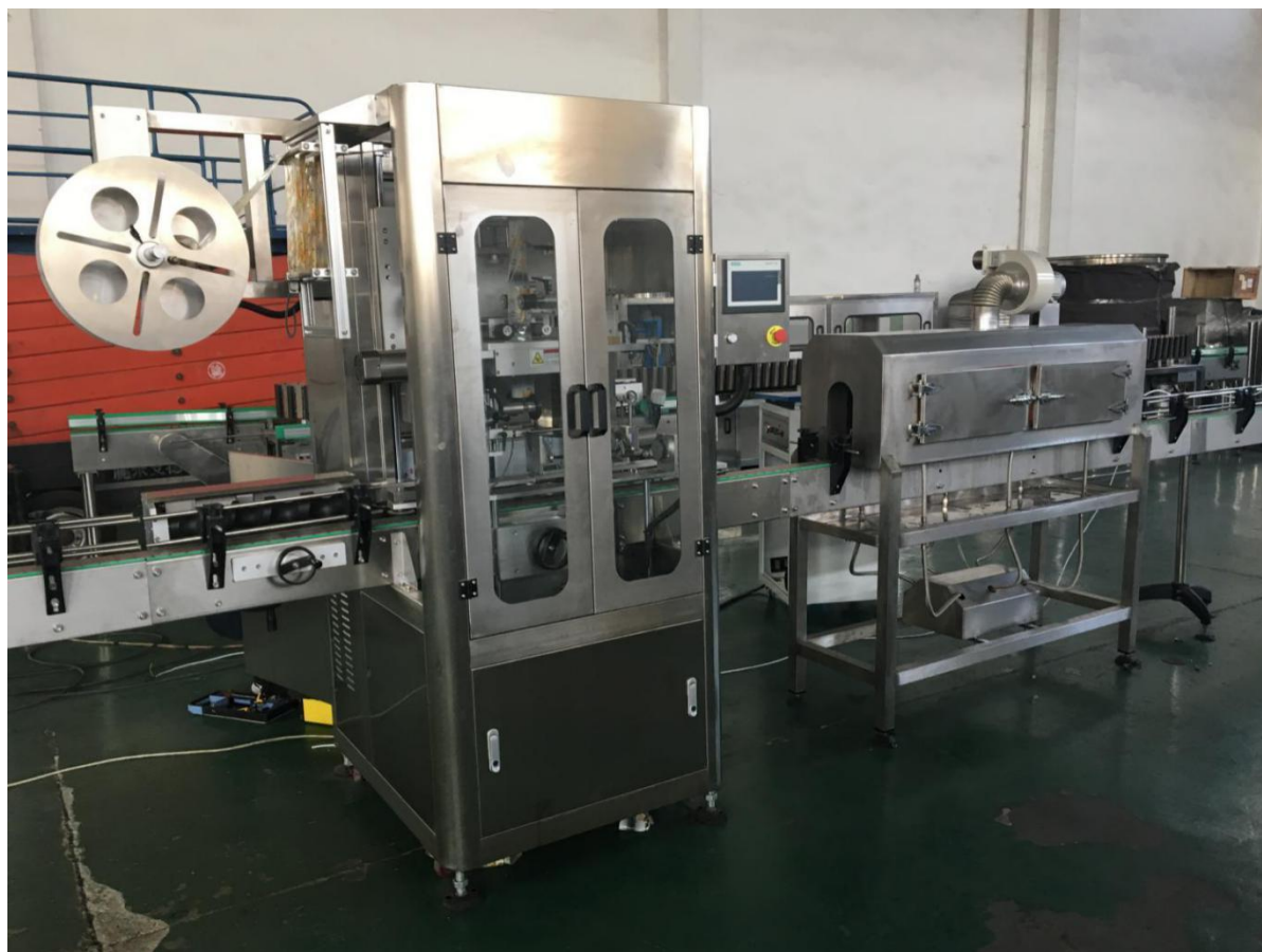
TB150 Labeling machine, shrink tunnel, steam generator connection for ref
