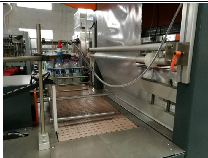
Bottle cylinder holding system to make sure one pack stability
